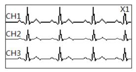
The LCD simultaneously displays the ECG waveform of three channels, and the right upper corner displays the current gain setting, and the left side displays the name of the corresponding lead (channel). (I, II, III, aVR, aVF, aVL, V1, V2, V3, V4, V5, V6, or CH1, CH2, CH3 under
