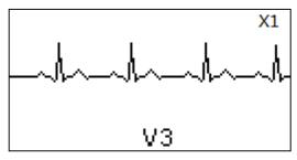
one-channel ECG wave, the right upper corner displays the current gain setting, while the bottom displays name of the lead (channel) ( I, II, III, aVR, aVF, aVL, V1, V2, V3, V4, V5, V6 or CH1, CH2, CH3 under 3-channel mode), Press right-up key ( ) or left-down key ( ) to change the ECG lead (channel), and press confirmation key ( ) to enter the next process.
